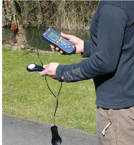
A sample image of using lux meter towards the sky.
